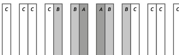
Figure 2. Example of class based storage - within aisle storage
