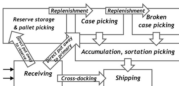
Figure 1. Typical warehouse functions and flows
